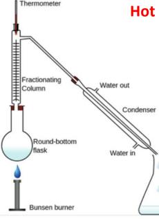
25°C FUEL GASES Cool C<sub>1</sub>-C<sub>4</sub> Calor gas, LPG 40°C GASOLINE petrol for cars 110°C NAPHTHA petrochemicals C---C-200°C KEROSENE jet fue C11-C1 300°C DIESEL (GAS OIL) fuel for diesel engine vaporised crude oil 350°C RESIDUE distilled further at lower > C<sub>20</sub> ressures to give FUEL OIL LUBRICATING OIL, WAXES and BITUMEN
